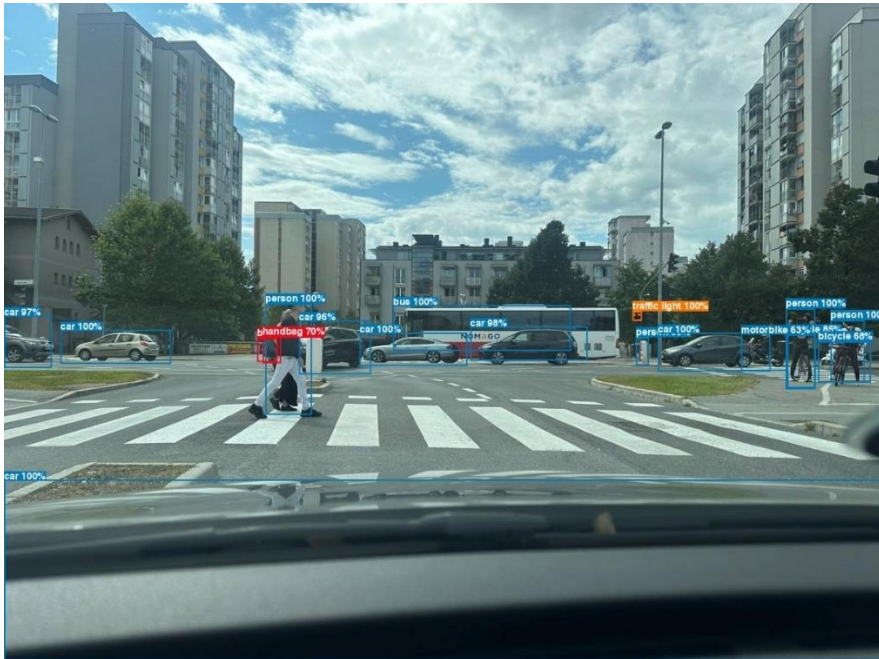
Figure 7 Object Detection using YOLOv5 Algorithm [19]
